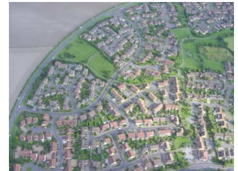
A contemporary single-use suburb with cul-de-sacs to avoid traffic and distributor roads to facilitate car use.
